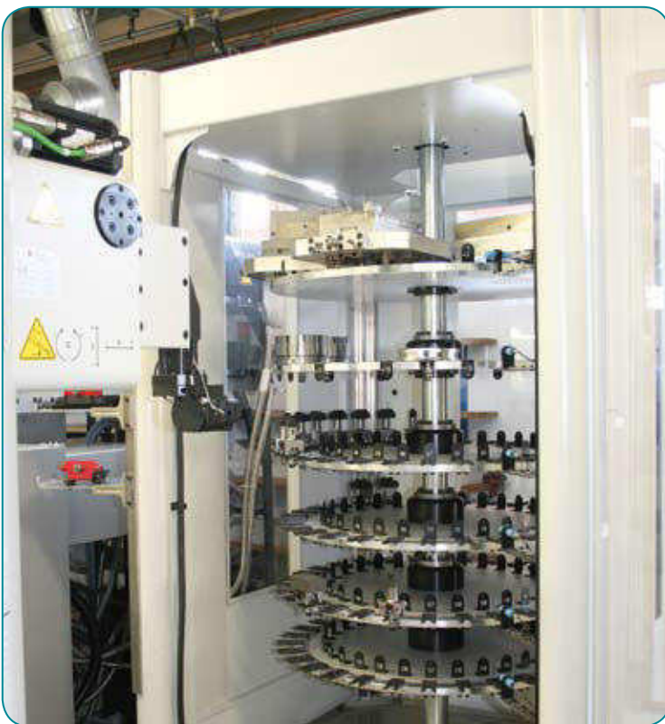
Magazine for palletising magnetic chucks and tools
