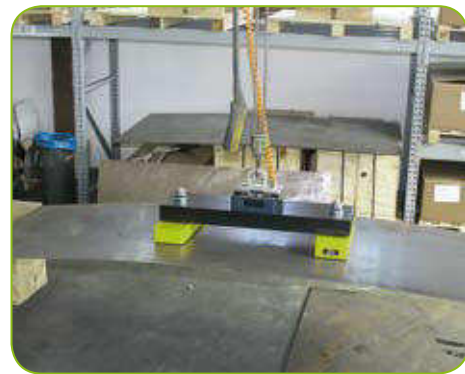
FXE-T to move thin sheet
