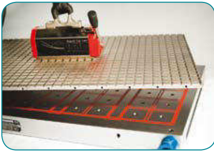
Step 1: Positioning the MAC VAC GRID adapter plate
