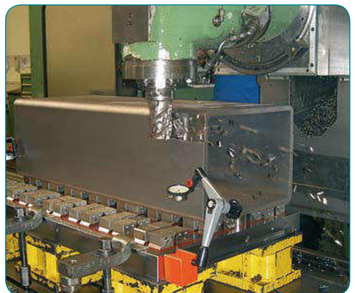
QX HD 50 with pole extensions for working with low vibrations
