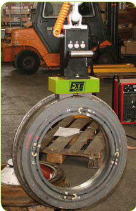
FXE with pole shoe for railway wheels
