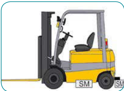
Tyre protection or Driveway cleaning on forklift
