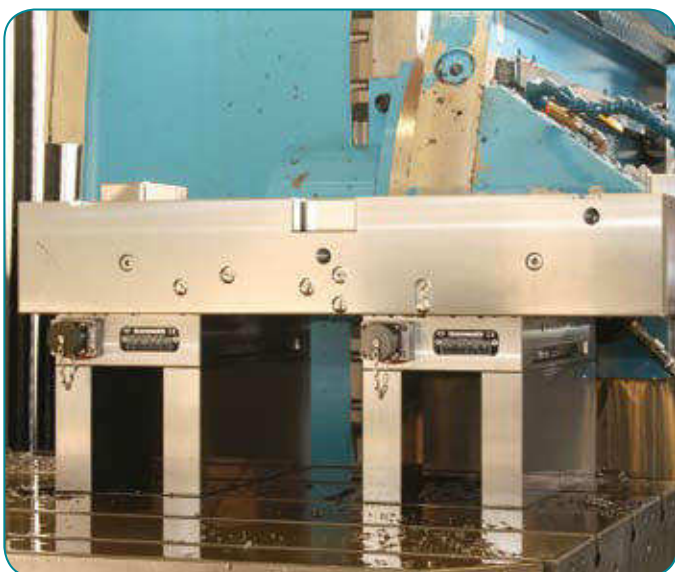
2 x QX HD 50 on columns for deep drilling
