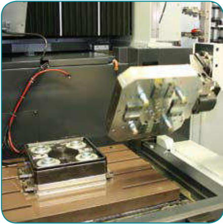
Assembly operation in an EDM machine with palletizing magnetic chucks system Erowa
