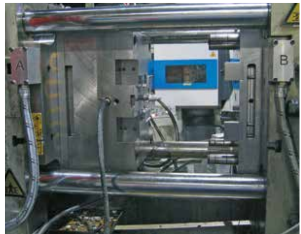
Magnetic clamping system on URPE die casting machine CC 125, closing force 1500 kN, magnetic force 110 kN, temperature range up to 240°C.
