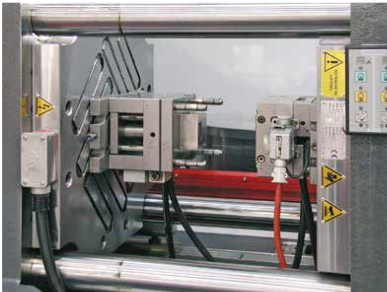
Magnetic clamping system on URPE die casting machine CC 125, closing force 1500 kN, magnetic force 110 kN, temperature range up to 240°C.
