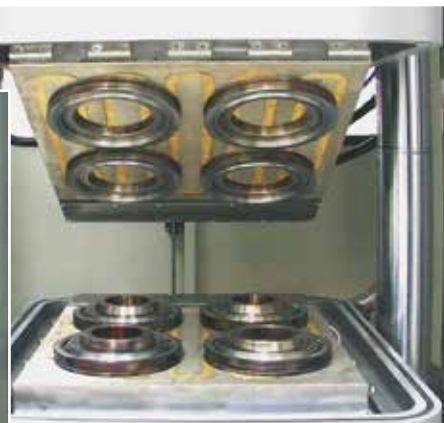
M-TECS 240 on a vertical press – various moulds on a machine bed without loss of space due to clamping claws
