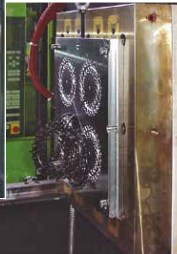
M-TECS 240 magnetic heating plate on an elastomer machine – full-surface magnetic force gives full-surface contact and more homogeneous temperatures
