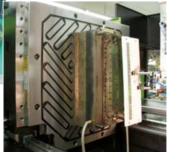
M-TECS 120 – An exceptional concentration of force: The magnetic force is transmitted through the long poles with double magnets into the clamping surface
