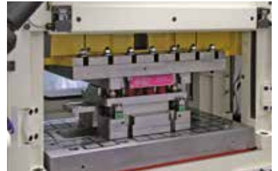
Magnetic clamping systems M-TECS 80 for sheet metal forming temperatures up to 80 °C
