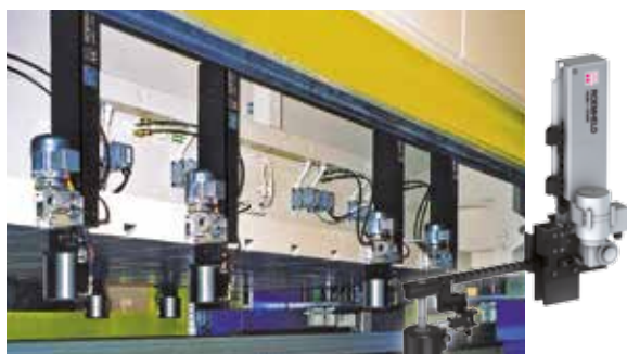
Electrical rapid clamping system with push chain fixed to the press ram of a double-column press
