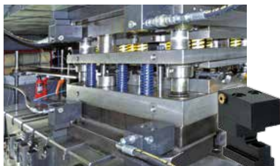
Sliding clamp with T-slot adapter in press bed and ram, roller bars and carrying consoles for tool insertion
