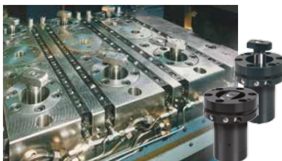
Swing sink clamps in a double-column press (tie rod extended in swing position)
