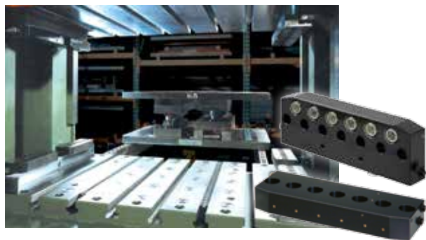
Clamping bars installed in press bed and ram. Easy feeding of dies by die change consoles and roller bars installed in the T-slots of the press bed.
