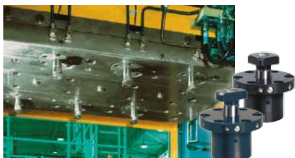
Swing clamps in the press ram. Die change position; ram in upper position, swing clamp extended
