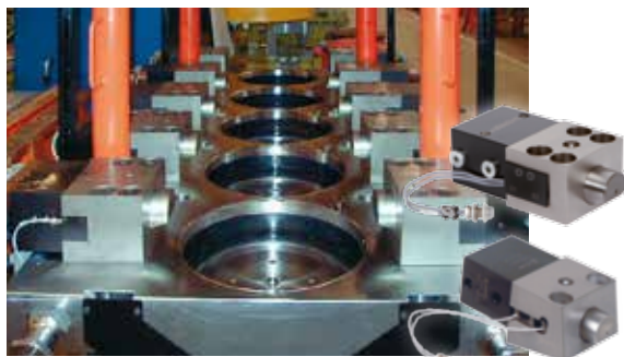
5-stage drop forge equipped with wedge clamps and directional control poppet valves to control the individual stages
