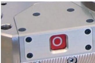
Optical clamping check, integrated into the fast closing clamp plate
