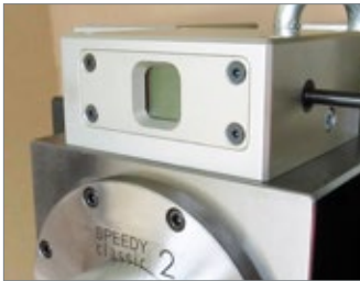
The green indicator indicates correct clamping.
