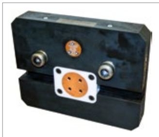
Example: Gripper and gripper plate for robot with multimedia coupling and electrically isolated ground terminal.
