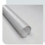
Transport Hose, extremely pressure/ vacuum-proof, smooth inner & outer linings, permanent antistatic, surface resistance < 10<sup>9</sup> Ohm, Food-grade quality (FDA/ EU 10/2011)
