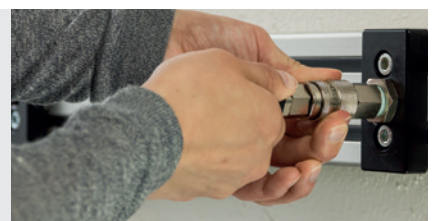
Two-hand operation: The disconnection is effected while pushing the plug and pulling back the sleeve
