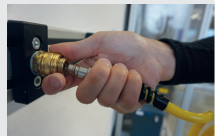
To disconnect pull back the sleeve of the coupling (ball or pin locking opens automatically and releases the plug)
