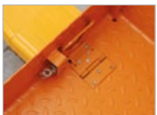
Security to prevent slipping from the straddle stacker
