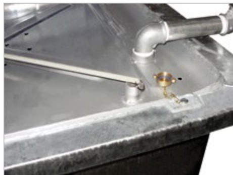
Dipstick to control the fill level
