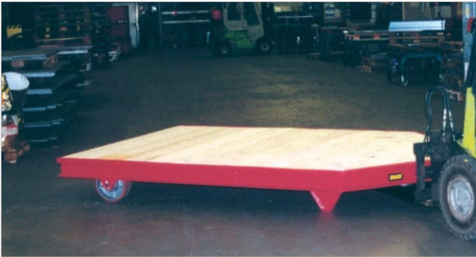
Drive the forks into the fork-sleeves of the STS, raise it and it is ready for use!
