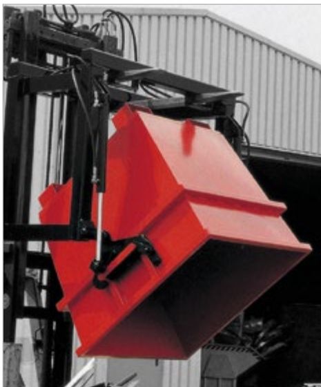
Type UC with pick-up feature for hydraulic traverse and hydraulic traverse type UCT
