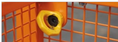
Anchorage point for protective equipment
