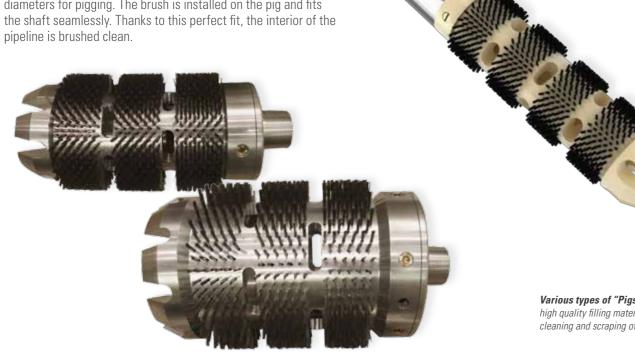
Various types of "Pigs" filled with high quality filling material for effective cleaning and scraping of the interior
