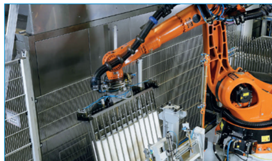
Gripping system for yogurt cups (varying diameters) / removal from deep-draw machine and packaging into boxes
