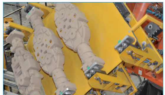
Gripping assembly system for sand cores / removal from core shooter
