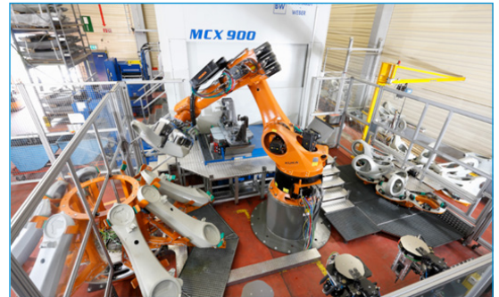
Gripper system, incl. tool changer for cast parts and deburring spindle / loading and unloading of machining center
