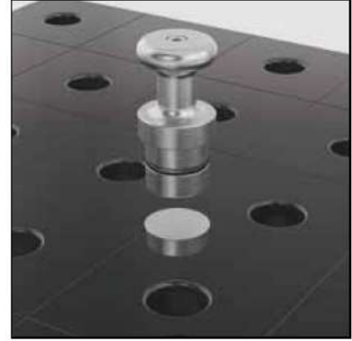
ill.: Removal of Cover Cap with magnetic clamping bolt
