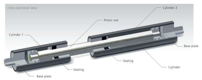
The special strength of HAHN Gasfedern is the solution of customer-specific tasks, for which we also develop unusual springs and products. The patent-protected double-stroke spring is an example for this.
