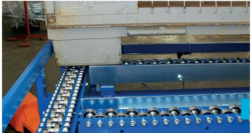
detailed view: side guide with deposit centering
