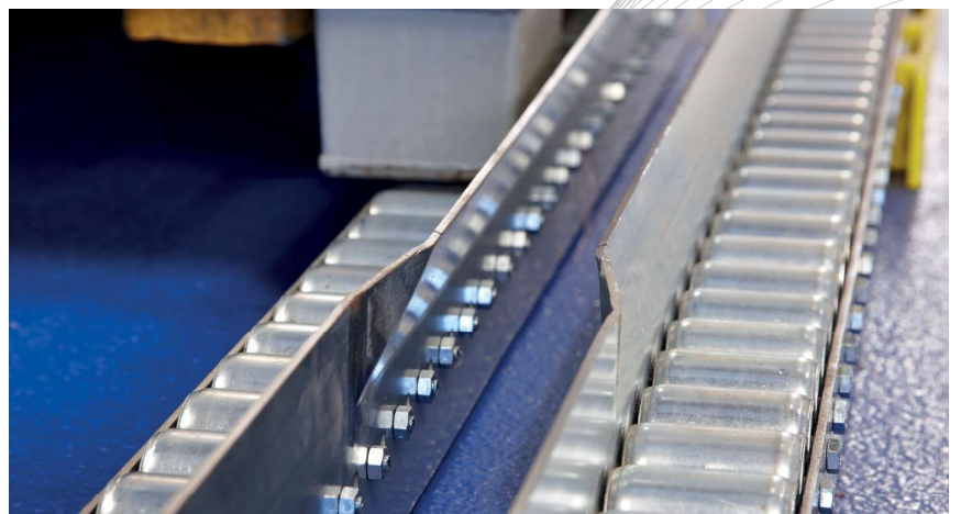
detailed view: side guide with deposit centering
