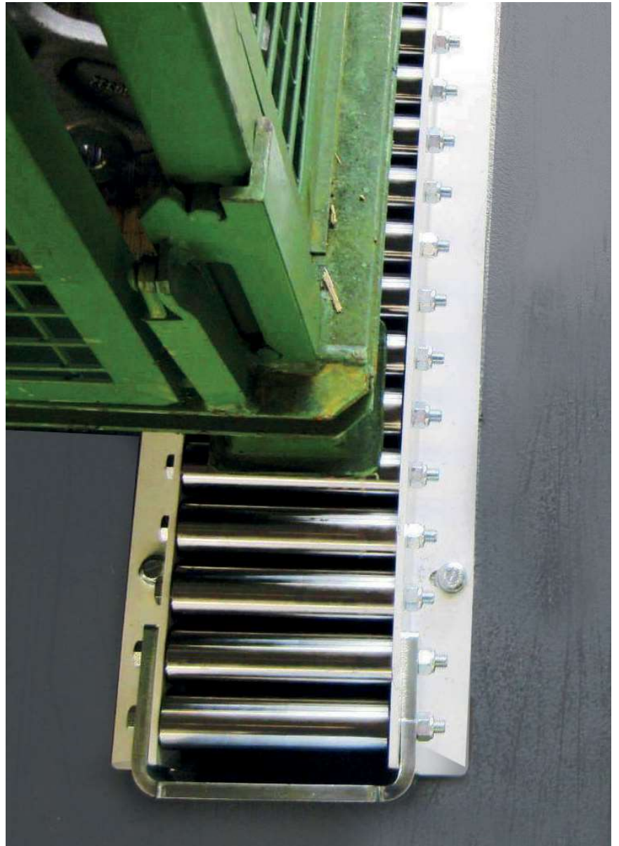
detailed view of the MTS with heavy-duty rollers
