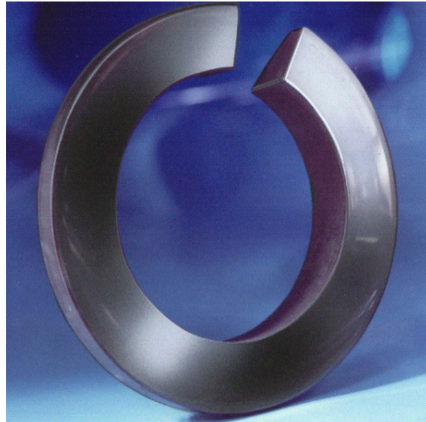
Fig. 11: Running surface of a carbon sealing ring after 10.000 hours of operation
