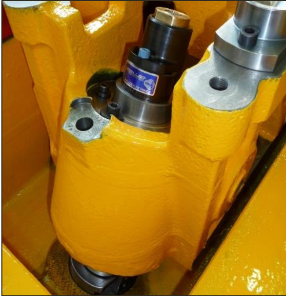
Pillar cam mounted in the blank holder in start position
