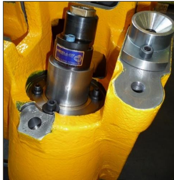
Pillar cam mounted in the blank holder in end position
