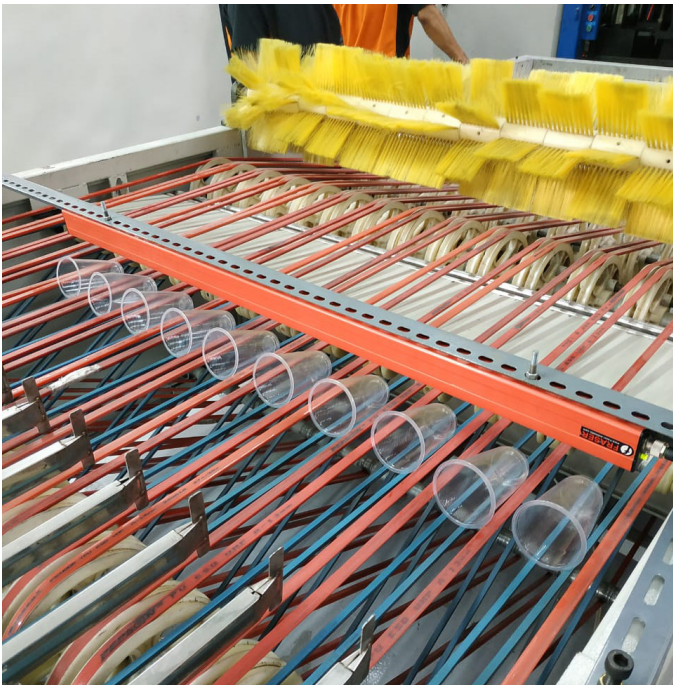
A NEOS 12F neutralising cups at the thermoformer output prior to stacking.
