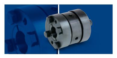
Rigid couplings with ultra-high torsional stiffness that were developed for servo motor applications. Unlike flexible couplings, they have no element to absorb differences between the centers of two shafts, so they have very high torsional stiffness. Since the outer diameter relative to torque can be reduced compared to flexible couplings, smaller couplings can be used, which helps reduce the moment of inertia.
