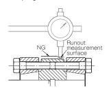
(4) Gently rotate the motor shaft manually and tighten the pressure bolt by adjusting it to make sure the value of dial gauge is zero.
