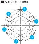
(5) Finally, use a calibrated torque wrench to tighten all the pressure bolts to the appropriate tightening torques of the table below, make sure that there is no bolts loosened and that the runout is small (the value almost near to zero), and tighten the driven shaft using the same procedure.
