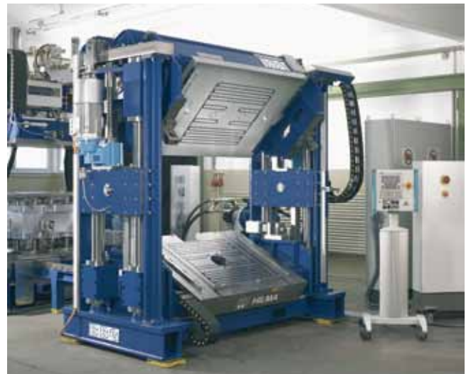
Magnetic clamping system for a mould carrier 1500 x 1000 mm, retention force 200 kN, temperature range up to 120 °C
