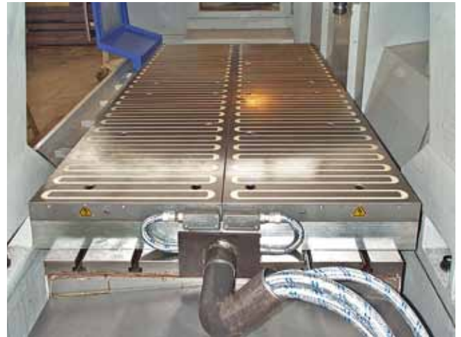
Long poles for heavy machining, plate size 2200 x 1200 mm with 2 connections, magnetic retention force 800 kN
