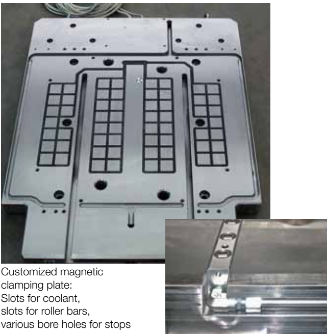
Magnetic clamping plate with square poles 70 x 70 mm, plate size 630 x 630 mm with lateral bore holes for stop bars
