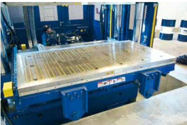
Magnetic clamping system for a sliding table 2500 x 1200 mm, retention force 800 kN, temperature range up to 230 °C
