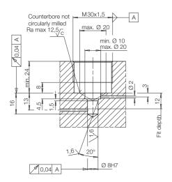
Threaded-body work support with threaded-body swing clamps as per data sheet B 1.891
