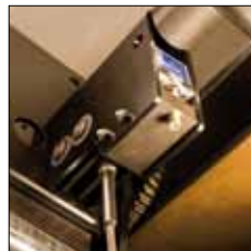
Overload prevention device prevents lifting excessive loads
