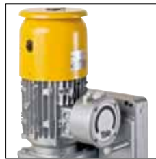
Hoist motor & brake Special motor with classification 1 Bm/M3 (1 Cm/M2 for 18 m/min) according to FEM/ISO 4301-1. Protected to IP 55.
