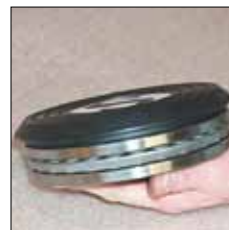
Ball bearing for turning plate
