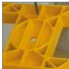
Chassis from ductile graphite iron
