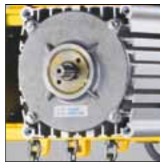
Externally adjustable slip clutch.
