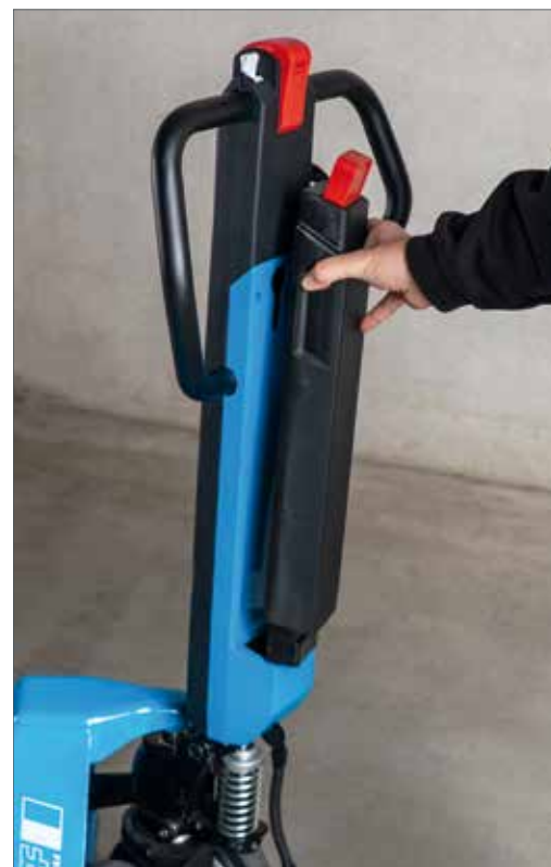
Fast battery change – with a single touch
