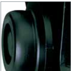
Wheel with cambered profile
