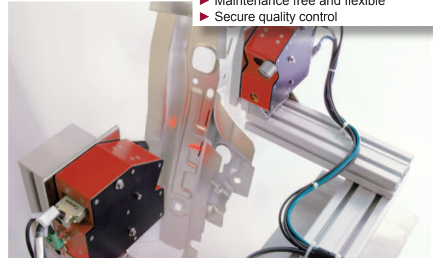
Weld Seam Geometry Inspection at automotive Components (Source: EHR®)
