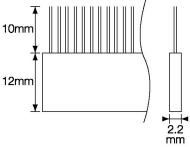
The brushes have a large number of highly conductive fibres. Positioned a few millimetres from the material to be neutralised, the fine tips of the fibre concentrate the electric field of the static charge and ionise the air. Ionised air provides ions of the opposite polarity to neutralise the static charge.
