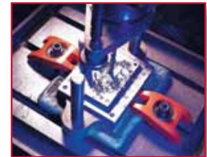
Working Height (H) Note that the bolt is always straight because of the swivelling pivot. Ranges from 0-75mm depending on model.
