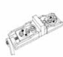
Unscrew traversing nut on moving head to allow jaw assembly to be moved forward.
