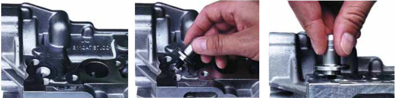
Mount retractable nipples (direct clamping of workpiece)
