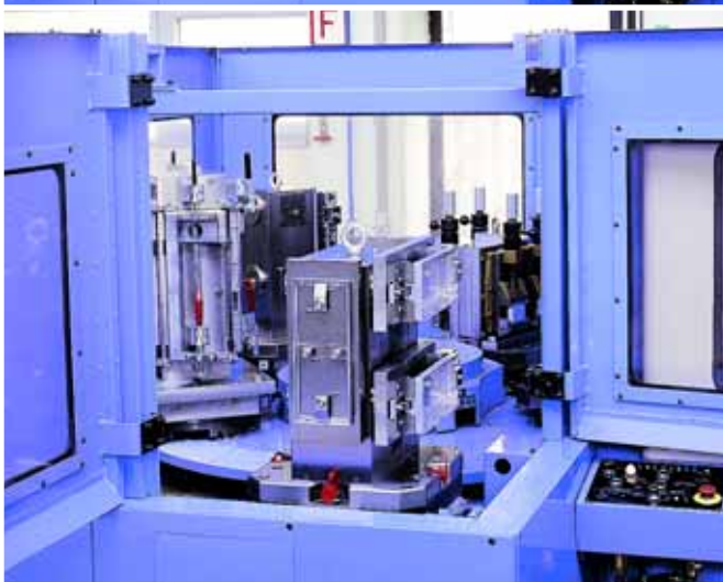
20 Setting up a machine centre with mounting towers.
