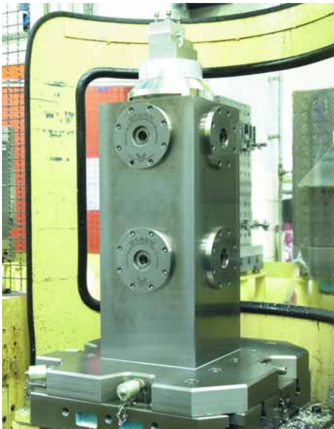
Pallet station with mounting towers, SPEEDY 1000 tubular set up and SPEEDY 1000 assembly
