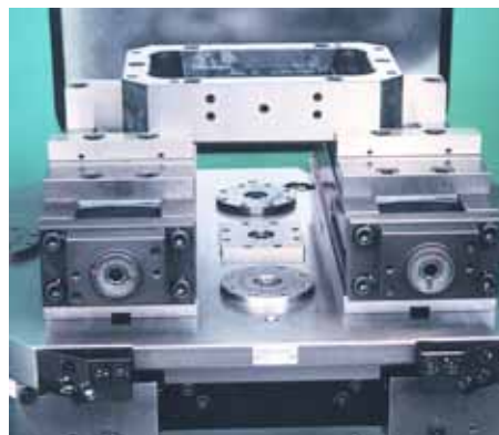
Machine pallet with a combined assembly of round and square SPEEDY clamps for central mounting.
