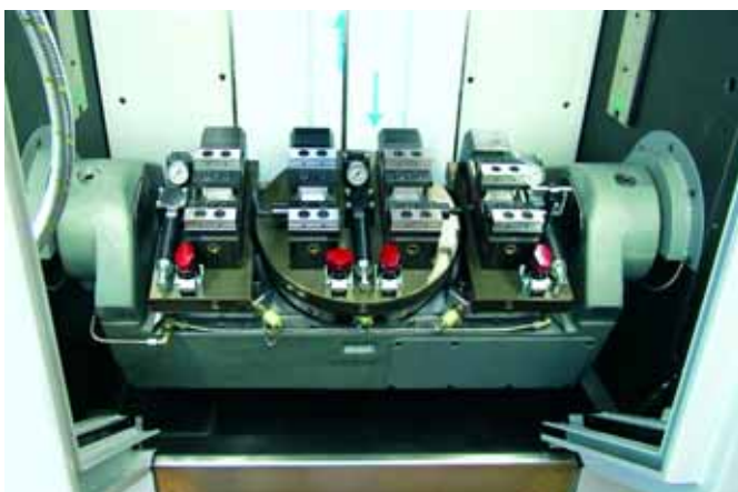
Rotation clamp device with 4 compact clamps. The compact built enables set up without collisions.
