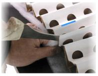
*Note:* you will cut through two paper layers (plus polyester in the HE). Pinch the pleats on either side beneath the knife for additional control while cutting.
