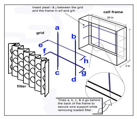
A one time installation of Andreae Wire Supports is necessary for the installation of Andreae pad size filters: 20 x 20 inch and 20 x 25 inch (51 x 51 cm and 50 x 63.5 cm).
