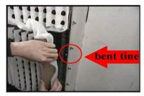
Slightly bend "bent tines" inward to allow space to tuck filter behind the tines. This is a one time adjustment. **Recommended**  $gap \simeq 1/8$  in (0.32 cm)
