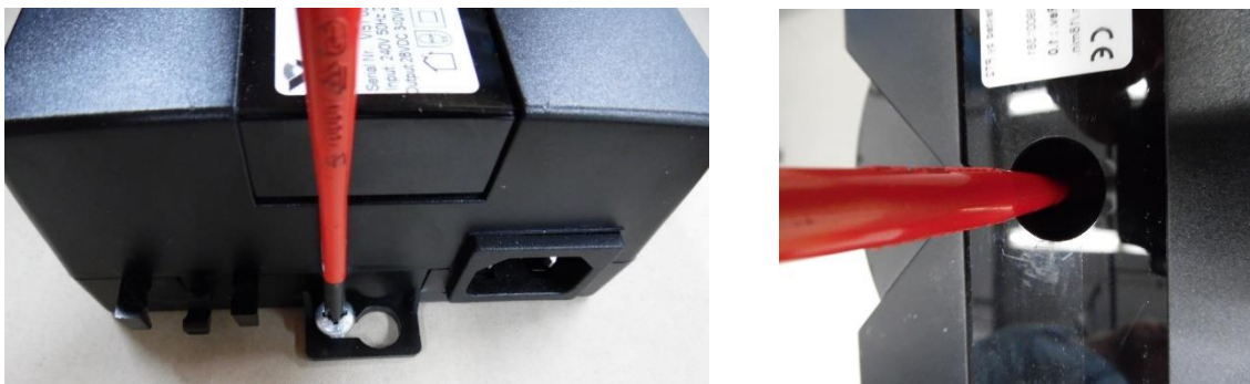
Figure 33 Mounting the electrical controller (Screw connection: left 3x, right 1x)
